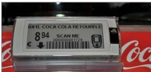
The Pricer DotMatrix labels offer a display with extremely clear information and high contrast. Their superiority in terms of readability is due to the use of real "E-paper technology" providing a wider angle of vision regardless of the lighting conditions.
